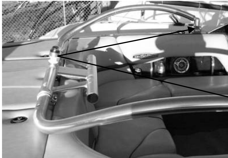
Figure 15 - Measure from ski tow to aft foot on each side
