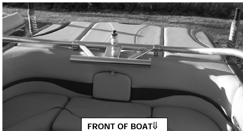
Figure 14 - Header and Aft Legs Lined Up
