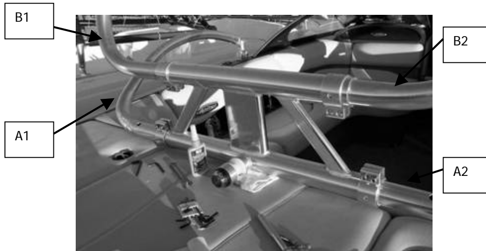
Figure 17- Header with Legs Attached
