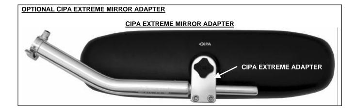
To use the OPTIONAL adapter for CIPA Extreme mirrors install the adapter to the end of the mirror mount instead of the mirror shown in the previous step. Loosen the cap screws to slide the adapter over the end of the mirror mount. By sliding the adapter in and out and using top or bottom mirror mounting options, the mirror can be adjusted to what suites you best.
