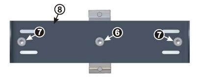
Make sure all bolts are tightened securely (15 ft-lbs) and we recommend using loctite on each thread to ensure they do not loosen from the vibration they will experience on the tower.
