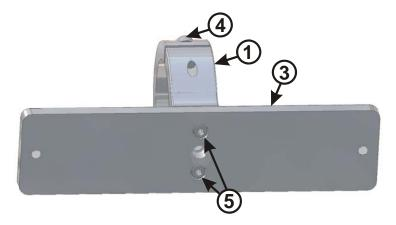
STEP 3: Attach the Kicker Speaker Bracket (Item 8) to the Speaker Plate (Item 3) using One M8x35 bolt (Item 6) in the center and Two M8x12 bolts (Item 7) as shown below.
