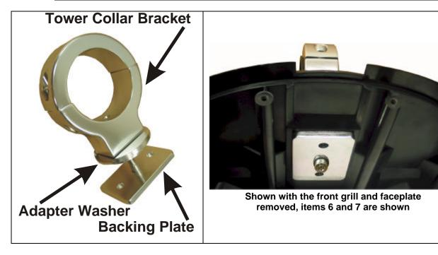
STEP 1: Determine if you are going to access the speaker from the front as shown above or by removing the wiring terminal on the back of the speaker shown below. It is much easier to remove the Rear Terminal Cover but it is more difficult to work from that access port.
