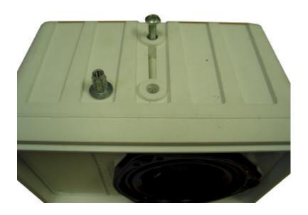
STEP 3: Remove the speaker by taking out the three screws holding it. At this point the top (front) hole will have the treaded insert ready to be removed, if it didn't drop into the speaker, in which case - hunt it down and eradicate it.
