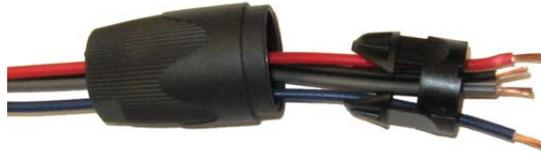
**Strip the ends of the wires, and tighten into the corresponding (+) and (-) sockets. Speaker wires are connected to 1+ and 1- Light connections are 2+ and 2- . Connector locations are marked next to the screws on the connector.**
