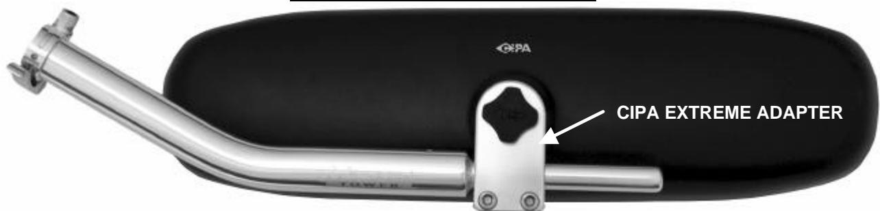
To use the **OPTIONAL** adapter for CIPA Extreme mirrors install the adapter to the end of the mirror mount instead of the mirror shown in the previous step. Loosen the cap screws to slide the adapter over the end of the mirror mount. By sliding the adapter in and out and using top or bottom mirror mounting options, the mirror can be adjusted to what suites you best.
