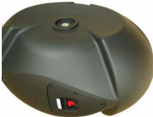
**STEP 2:** Once you have access to the inside of the speaker remove the bolt on the inside that is holding the treaded insert. This threaded insert is shown on the top of the speaker in the above photo. Note that for the other speaker you will remove the treaded insert on the opposite side.
