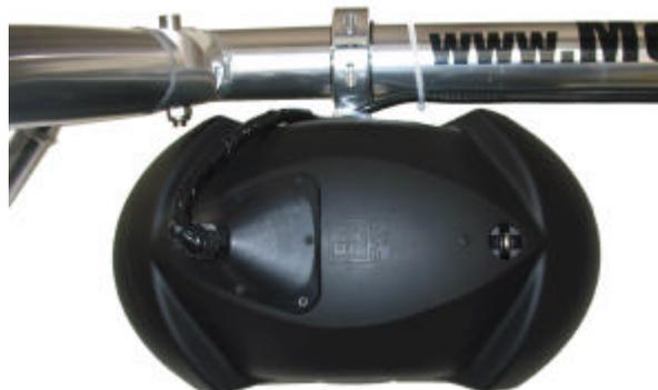
A small amount of rotation of the speaker is available to point the speaker towards the outside of the wake. This should be set once and not continually moved or you may need to retighten the M8x50 bolt inside the speaker.
