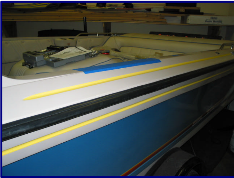
Figure 2 - Masking Tape on Deck
